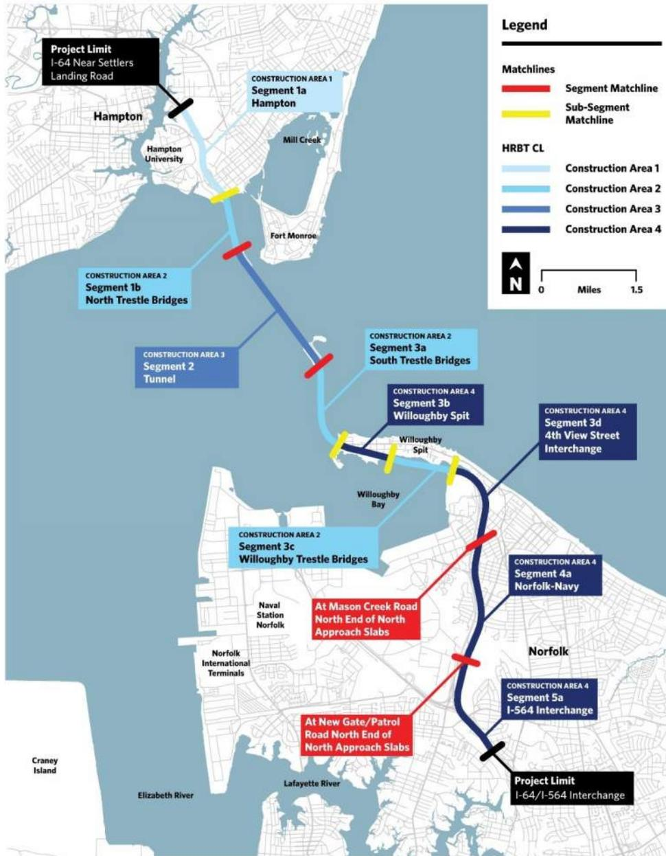
Figure T-1: HRBT Design Segments and Key Map
