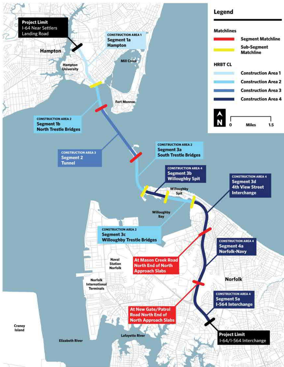
Figure I-1: HRBT Expansion Project Segment Map
