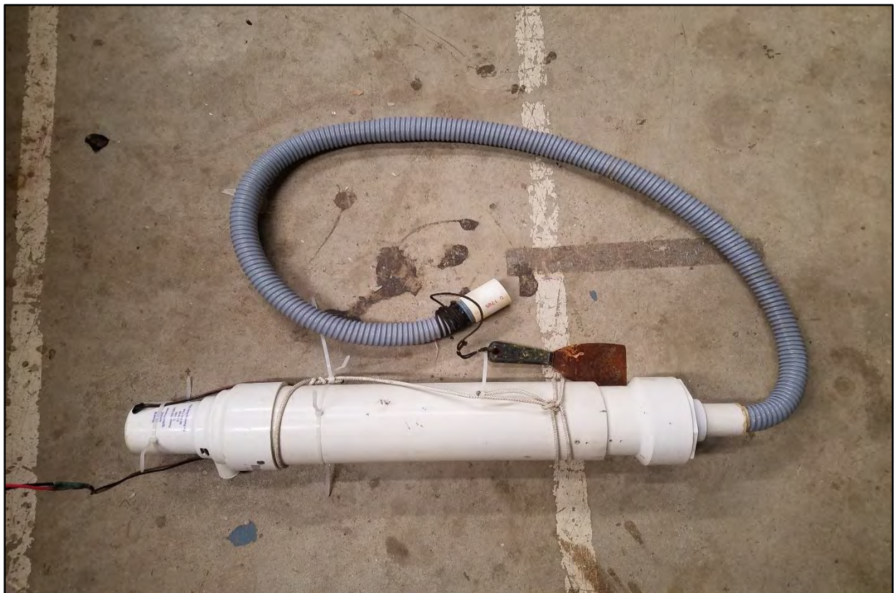
Figure 6. The Custom Suction Sampler Used to Sample the Rocky Shore of the Portal Islands
